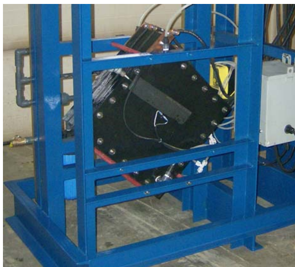
Containerless Graphite Electrolysis Cell
