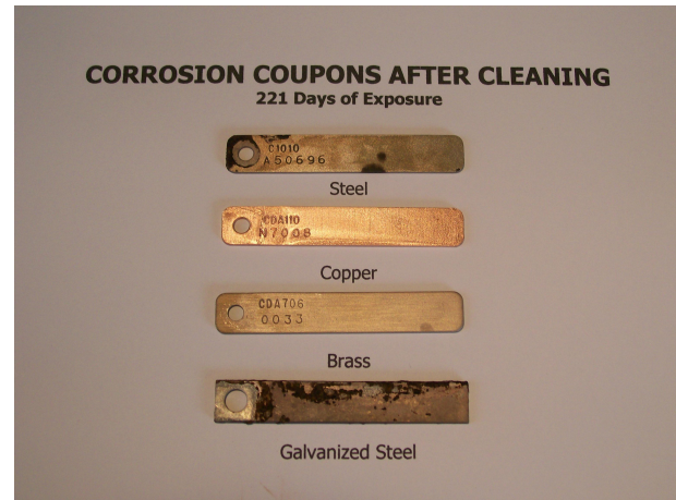
Photo 2: Corrosion coupons removed from soft water tower; light cleaning
