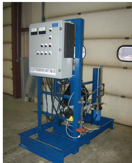
ElectroBrom Model EB-30 30 lb/day bromine production
