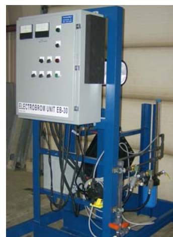
Electrolytic Bromine Unit
